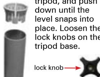
**4** Slide legs toward or away from the base until the bubble rests in the center of the bubble level. The tripod is now level. Tighten the lock knobs, and remove the bubble level.
