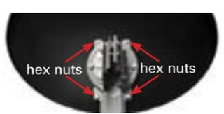
**8** If two carriage bolts were added to the two additional skew holes, loosen and remove the two carriage bolts and the two hex nuts.
